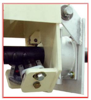
The model RKS front lance support roller assemblies are constructed using dual roller bearings with a hardened roller wheel. The bearings are sealed; however, grease fittings are provided for periodic greasing due to extreme heat operating conditions. The roller brackets are offset so that the rollers can track on a perfect angle to the lance. The roller assemblies can be easily adjustable if required.
