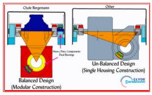
The dual rack-&-pinion drive has been developed using a "Balanced Design" concept. All major components such as the poppet valve, feed tube, traveling carriage and lance tube are symmetrically located on the centerline of the sootblower housing. This "Balanced Design" construction evenly distributes the forces caused by pressurized cleaning medium over the drive train thus minimizing gear, pinion and rack wear.
