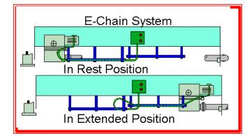
The unique "E-Chain" power supply assembly provides electrical power from the stationary junction box to the traveling carriage assembly. This system has proven to be dependable, low maintenance and durable in the most severe operating conditions.
