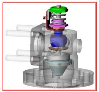
The poppet valve is a mechanical design and has a removable seat and disc assembly for ease of repair. A pressure control orifice is provided so the blowing pressure is adjusted independent from the valve opening. The pressure adjustment is made external to the poppet valve and while the sootblower is in operation. This allows for very precise adjustments, improved safety and quick adjustment.
